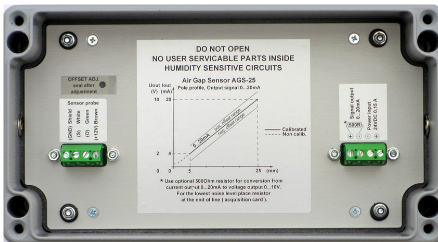
Figure 20. AGS Signal Conditioner unit enclosure with cable inlets (CAB) (after S/N 144701)
