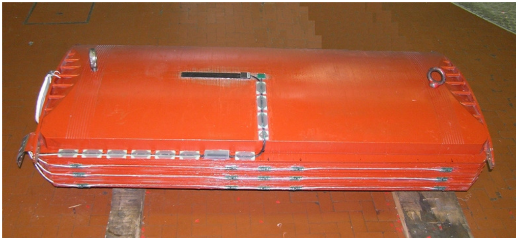
Figure 27. AGSP sensor probe installed at rotor pole (AGSP sensor pictured next to Magnetic field sensor in the middle of rotor pole)
