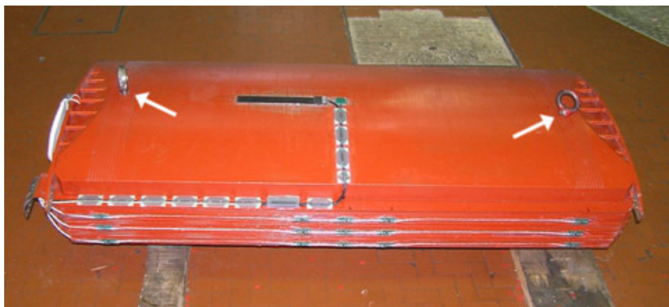
Figure 5: Rotor pole, arrow showing positions of pole lifting hoist attachments
